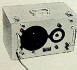
NF Signal-Generator (Western Electric Oscillator 19 C/SPL).
